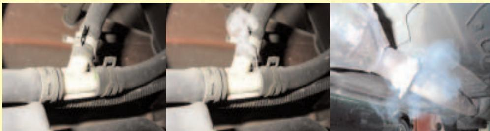
It is impossible for the human eye to tell the difference between a 0.020-inch and a 0.040-inch leak opening, and in some cases even find that elusive leak at all. A diagnostic smoke machine is recommended equipment for effective EVAP emissions diagnosis.
